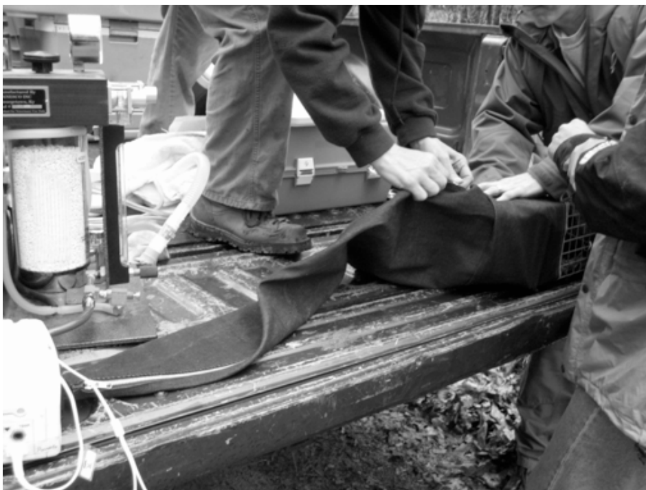
Figure 5. (b) The denim cone shown wrapped around the cage front and tightened with heavy duty Velcro.
