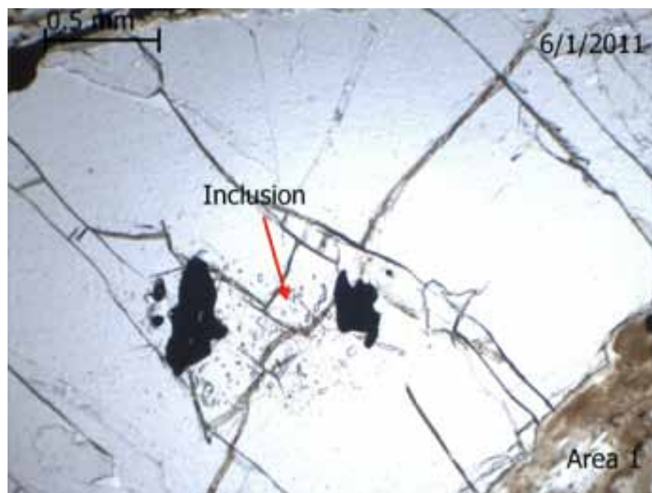
Figure 4: Photomicrographs showing a garnet grain in plain polarized light with inclusions in the center of the grain and the tail of the grain. The arrows in the left photo indicate the orientation of sillimanite inclusions. The area encompassed by red in the right photos shows the inclusion rich garnet core.
