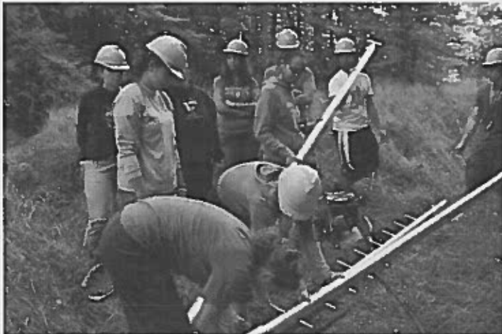
Students in environmental geology assemble the vibracoring tripod in preparation to take a core (P. Colgan).
