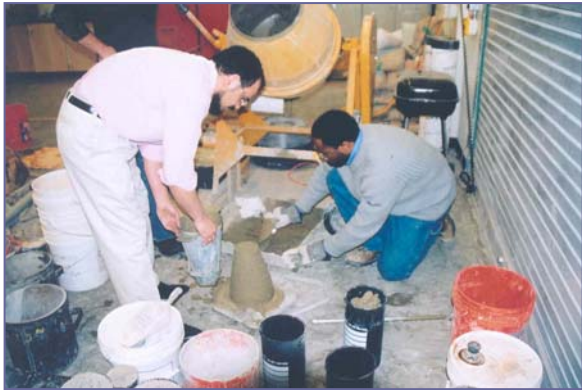
Antwan (right) and Dr. Sherif Yehia, Ph.D., working in a lab to slump test freshly mixed high volume fly ash concrete.
