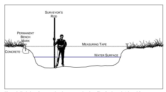
Figure 8: Technique for measuring the cross-sectional profile of a channel. Adapted from Rosgen (1996).
