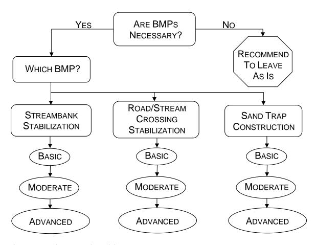
Figure 1: Erosion Control Decision Tree
