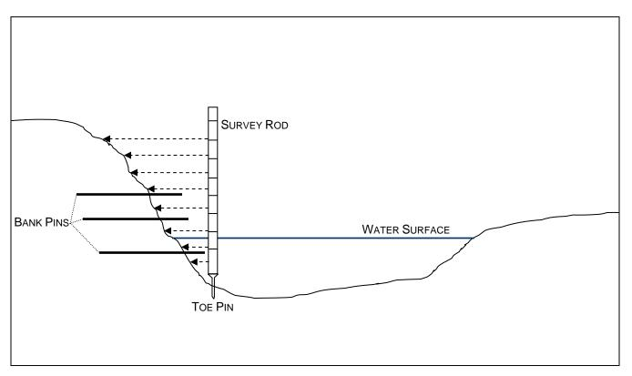
Figure 6: Example of bank pin placement and bank profile measurement. The arrows indicate measurement points for the bank profile. Modified from Rosgen (1996).
