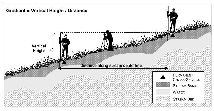
Figure 7: Longitudinal cross-sectional view of a stream, demonstrating the technique for measuring the longitudinal profile of a channel. The riffle-to-riffle gradient is an approximation of the average water surface slope of the reach. Adapted from Rosgen (1996).
