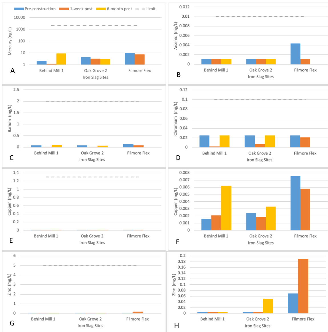
Figure 5. Metals for pre- and 1-week and 6-month post construction. Blue is pre-construction, orange 1-week post construction, yellow 6-month post construction. The grey dotted line represents the drinking water standard for either EPA or WHO which ever was the smaller of the two standards for the given chemical. The legend in A applies to B-H. F and H are enlarged versions of E and G respectively.
