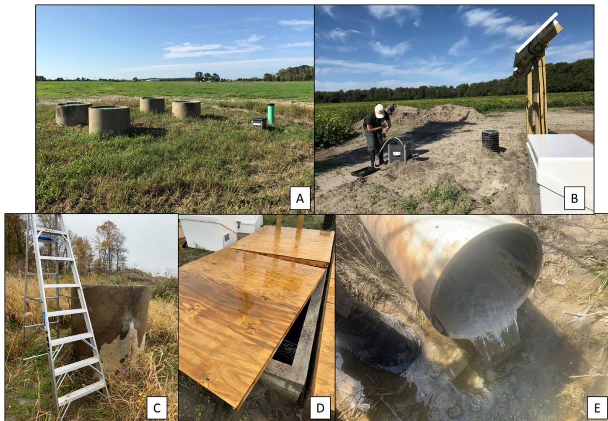
Figure 4. Photos of different sampling locations. A) Behind Mill 1 with completed iron slag filter in place. The green tube (far right) is an inflow sampling port that was installed only at this location. Access ports (four cement upright tubes with green caps) are for two slag filters which receive tile drain water from the adjoining field (in background) and used to sample outflow. B) Research Assistant, Emily Kindervater, using a hand pump siphon to sample from a below-ground control box (inflow) at Filmore Flex; Oak Grove 2 has a similarly constructed inflow (not shown). C) Slag filter outflow access point for Oak Grove 2, which required a ladder to removing the large plastic green cap and accessing filters. D) Slag filter outflow access point from Filmore Flex in which is covered with large plywood lids. E) Outflow pipe at Behind Mill 1; the white particulate residue inside the tube is from a calcium carbonate layer placed on top of the iron slag inside the tanks to balance pH.
