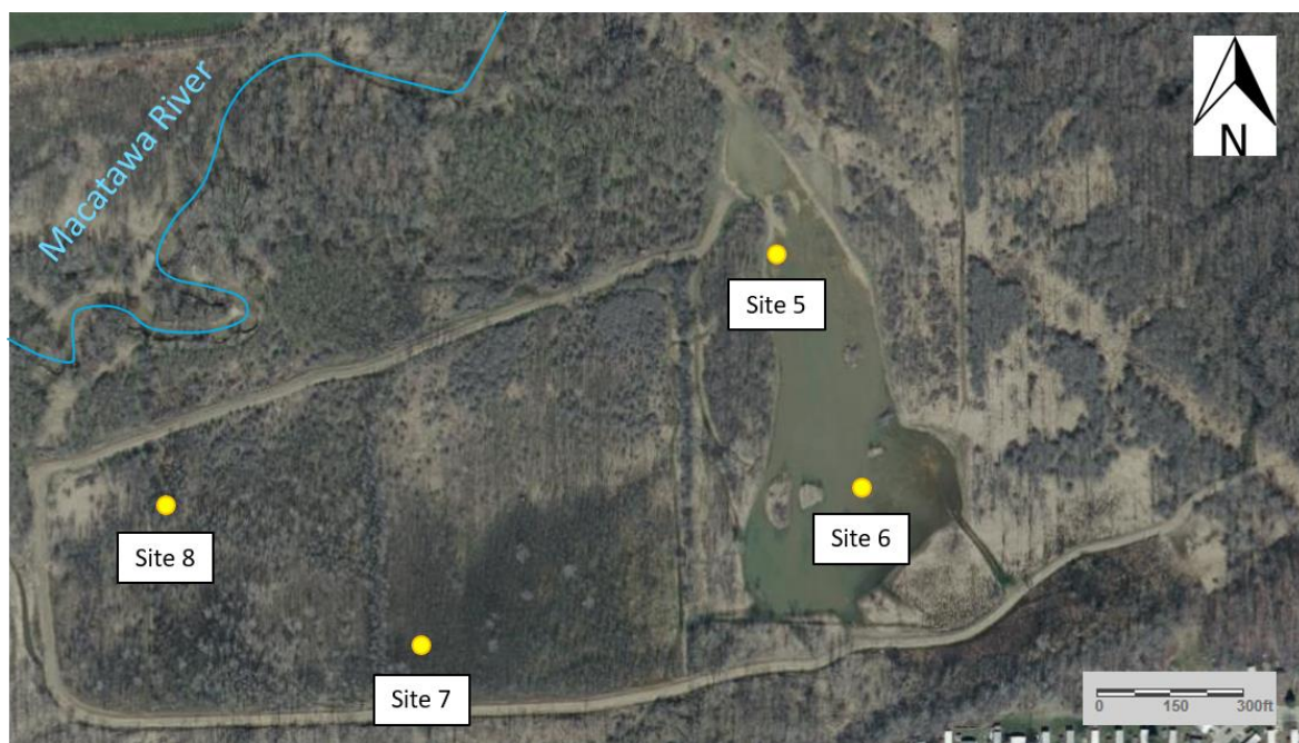
Figure 3. Middle Macatawa wetland sediment coring sites (n=4 total; sites 5, 6 are in the excavated restoration area and sites 7, 8 are in the unexcavated area).
