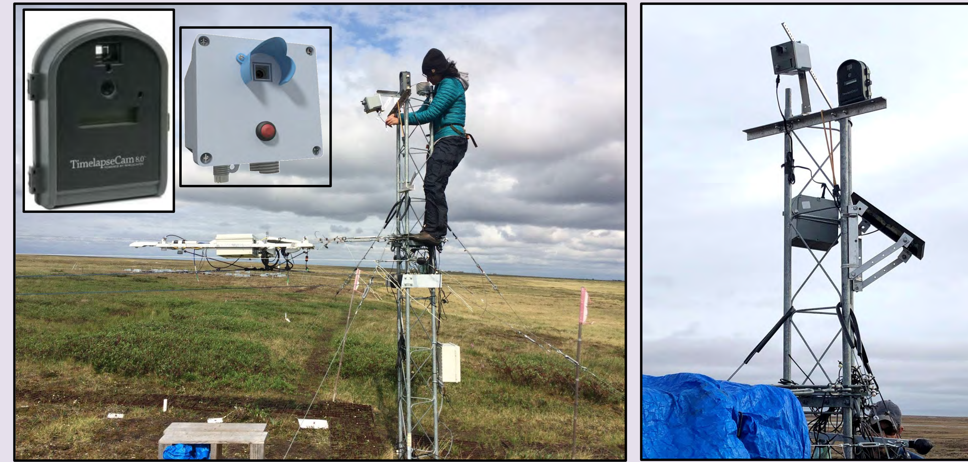
Fig. 3. Phenocams were installed on top of the MISP transect towers at both Utqiagvik and Atqasuk, Alaska during summer of 2011 and 2016. The Wingscapes Birdcam and UTEP proprietary camera models were used and programmed to capture hourly images throughout each growing season.
