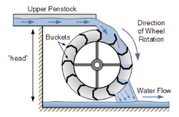
An overshot wheel includes a vertical wheel with a horizontal axle. A typical overshot wheel has the water channelled to the wheel at the top and slightly beyond the axle. The water collects in the buckets on that side of the wheel, making it heavier than the other "empty" side. The weight turns the wheel, and the water flows out into the tailwater when the wheel rotates enough to invert the buckets. The overshot design is very efficient, it can achieve 90%, and does not require rapid flow.
