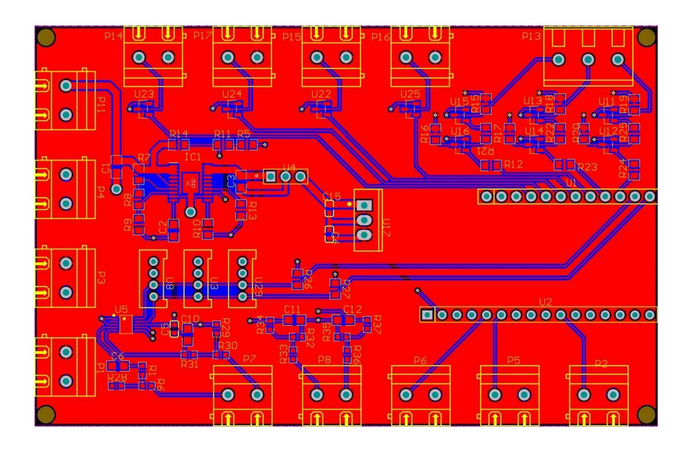
The ESP32 microcontroller is used to control the system. The ADS1115 is used to perform analog to digital conversion on the test and reference sensors. The ESP32 is connected to WiFi and it communicates to AWS via the AWS IoT Core. The GUI unlizes a custom API that interfaces with the ESP32 and the machine. AWS Lambda Functions are utilized to send test results to a database.
