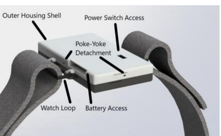
The Band Mounted Accelerometer provides force feedback through acceleration data. Bands will be strapped to the user's
